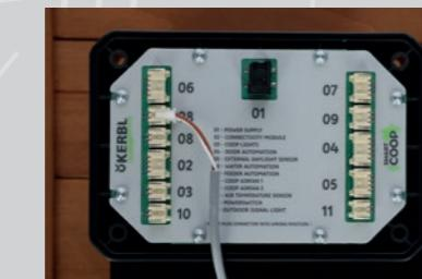
If the connection cable built into the module is not long enough, it can be lengthened using extension cables (items 70629, 70630). Ensure that the connection location is protected from water and dust. The module cable must have only a single extension.
